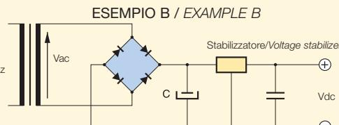
The supply voltage should be adjusted according to the characteristics of the sensor used. It is recommended to use a transformer with secondary voltage Vac lower than the direct voltage Vdc required. The secondary voltage Vac is found as follows:
